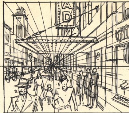
ONE VANISHING POINT PERSPECTIVE TAKE A POINT ON THE HORIZON, DRAW RADIATING LINES IN ALL DIRECTIONS FROM IT. YOU CAN NOW BUILD ON THOSE LINES BY CHOICE. OF COURSE YOU NEED TO KNOW PERSPECTIVE TO DO IT.
